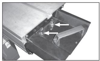
Figure 1. New sliding table handle with two lock handles.
